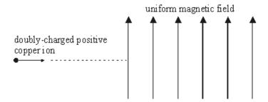
The diagram above shows a doubly-charged positive ion of the copper isotope  $^{63}_{29}$  Cu that is projected into a vertical magnetic field of flux density 0.28 T, with the field directed upwards. The ion enters the field at a speed of  $7.8 \times 10^5$  m s<sup>-1</sup>.
